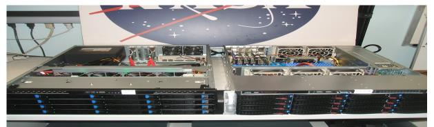
Figure: Right case houses Core i7 cores, DDR3 memory, NIC, two "internal" controllers each with eight disks and two "external" controllers; left case houses sixteen SAS-connected disks.
