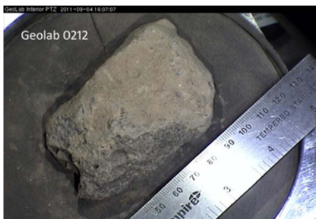
Fig. 3. Image of rock sample 0212 processed in the Geolab and analyzed by VAPoR. Sample 0212 is a vesicular basalt fragment covered with light brown soil with a total mass of 156 g (photo credit: NASA).
