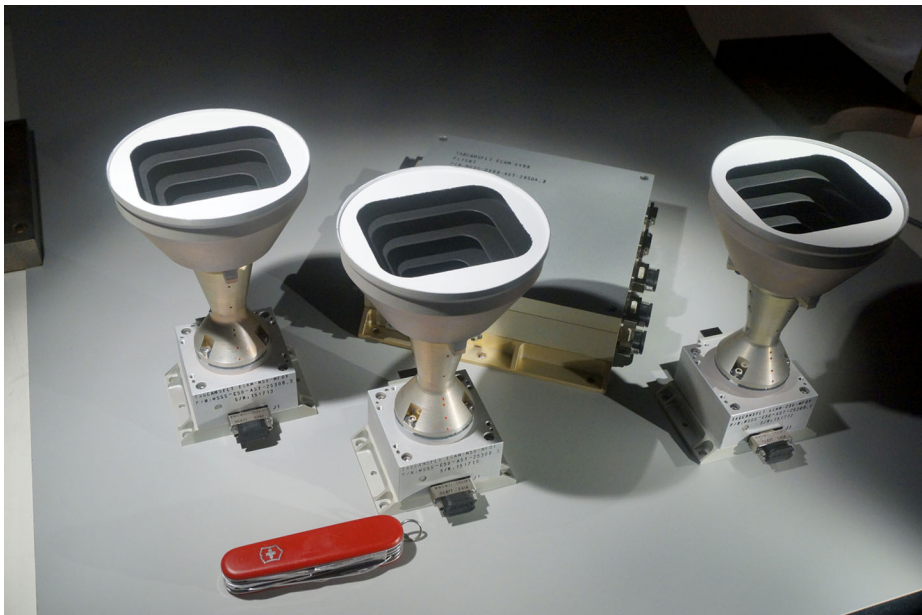
Fig. 19 The TAGCAMS flight unit built by Malin Space Science Systems. The two Navcams are at the left and center and the Stowcam is on the right. The digital video recorder is behind the center camera head, containing two separate recorder boards. The pocketknife is for scale (Malin Space Science Systems)
