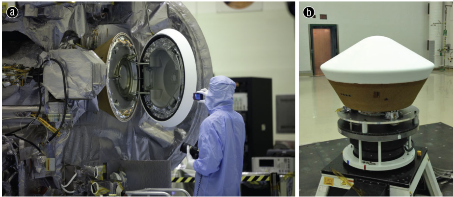
Fig. 13 The Sample Return Capsule is the only part of the OSIRIS-REx spacecraft that will return to Earth at the end of the mission. (a) A technician inspects the open capsule during testing. (b) The closed SRC sits in a Lockheed Martin cleanroom (Lockheed Martin)
