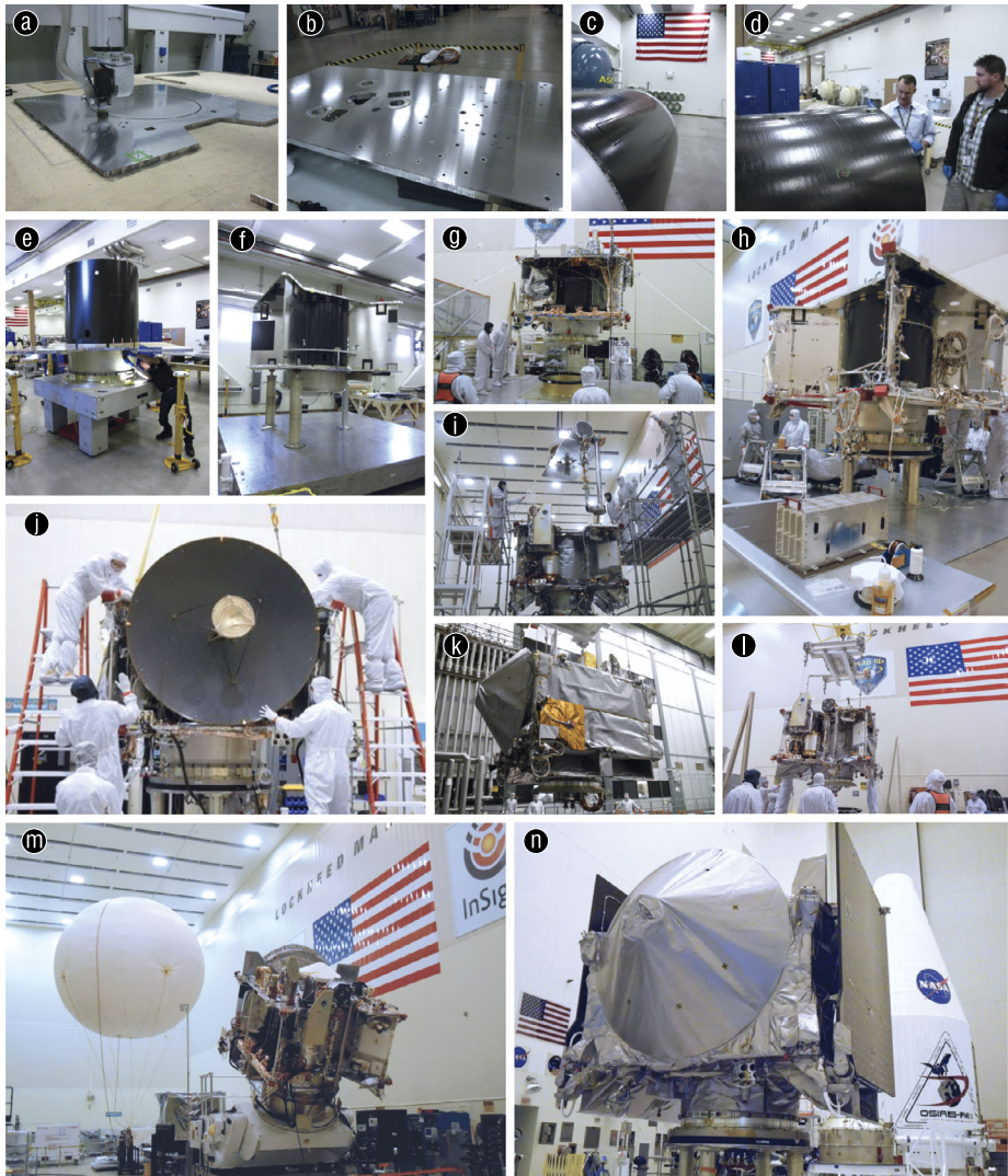
Fig. 10 Progression of the OSIRIS-REx spacecraft's assembly at Lockheed Martin Space Systems in Littleton, Colo. (a) Final machining of the Aft Deck on the 5-axis router. (b) SARA panel post machining spool and insert bonding. (c) The first flight hardware built in manufacturing, the composite sandwich structure of the core cylinder after cure, ready for machining. (d) Mission Principal Investigator Dr. Dante Lauretta and Lockheed Martin ATLO Floor Manager Ben Bryan inspect the core cylinder before assembly. (e) Structural assembly of the aft deck and alignment with the core cylinder. Alignments and assembly work are done on a flat granite table. (f) Composite structure assembly post-alignment verification, ready for static testing. (g) Lifting the assembly to the rotation fixture for initial testing. (h) First operations in ATLO, the harness routing and installation. (i) Final SARA/TAGSAM installation. (j) Final HGA installation and alignment. (k) Lifting spacecraft into the Lockheed Martin Thermal Vacuum Chamber for Environmental testing. (l) Lifting spacecraft into the shipping container in preparation for transport to NASA Kennedy Space Center in Cape Canaveral, Fla. (m) Completed spacecraft installed on a rotation fixture at Lockheed Martin Space Systems. The balloon in the background was used to simulate weightlessness during testing of the TAGSAM arm. (n) Completed spacecraft prior to fairing encapsulation in the NASA KSC Payload Hazardous Servicing Facility (Lockheed Martin)
