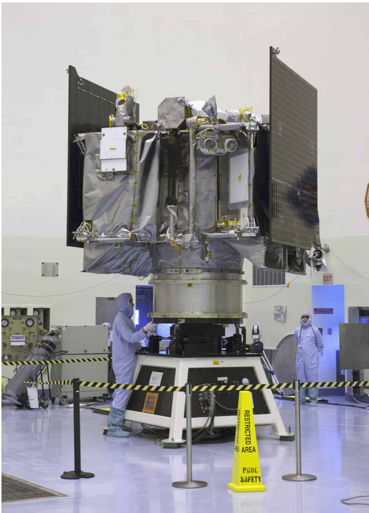
Fig. 8 The OSIRIS-REx spacecraft installed on a rotation fixture in a NASA Kennedy Space Center cleanroom in preparation for launch (NASA)
