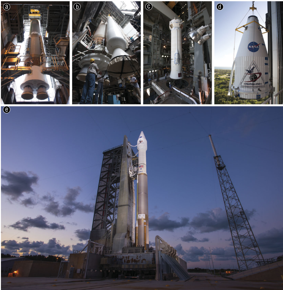
Fig. 24 United Launch Alliance provided the OSIRIS-REx launch vehicle, an Atlas V 411 rocket. (a) A crane lifts the Atlas V rocket's first stage booster, placing it into position at Space Launch Complex 41 at Cape Canaveral Air Force Station (NASA). (b) Team members guide the solid rocket motor into position for attachment to the Atlas V rocket's first stage booster at Space Launch Complex 41 (NASA). (c) Team members prepare to attach the Centaur upper stage to the Atlas V rocket's first stage booster (NASA). (d) The OSIRIS-REx spacecraft, encapsulated in its fairing, is lifted to the top of the Atlas V rocket assembly (NASA). (e) The OSIRIS-REx mission's Atlas V rocket is ready for launch on Launch Complex 41 (United Launch Alliance)
