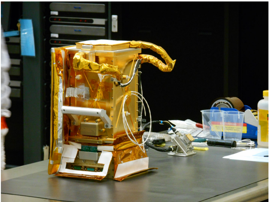
Fig. 18 The Regolith X-ray Imaging Spectrometer (REXIS), a student-built instrument, will determine which elements are present on the surface of Bennu (MIT)
